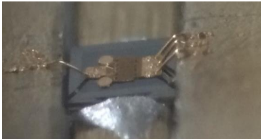
Fig.1. Connecting the transistor to the substrate using wire bonds.
