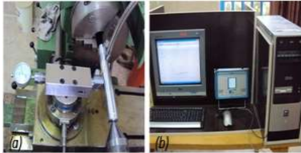
Fig. 3 Analog-to-digital dynamometer converter and display screen, with the workpiece secured in the device for the burnishing process.
