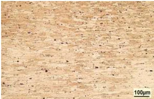
**Fig. 4** Optical micrograph of the AA7075 base metal.
