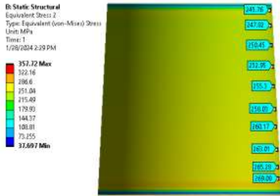
Fig. 16 The value of stress in different radii of the cone.
