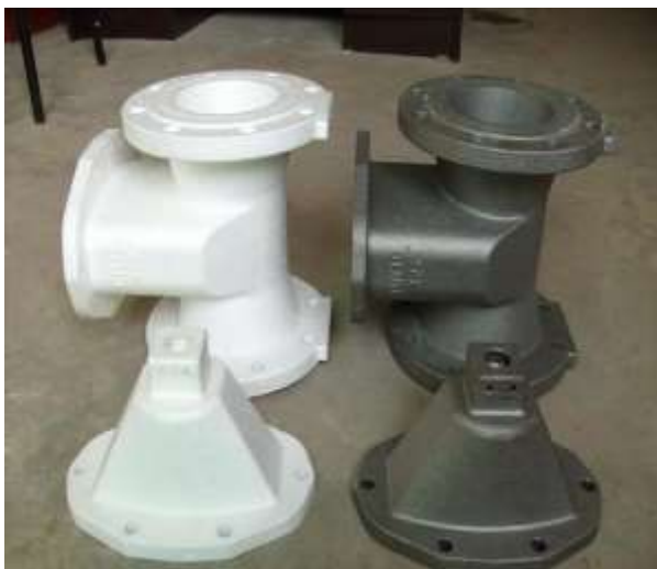
Fig. 1 Complex piece produced by the lost foam method.
