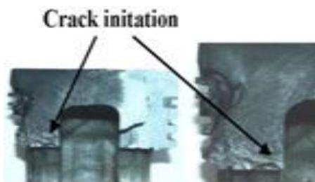
Fig. 15 A cracked engine piston in upper portion of piston pin [34].
