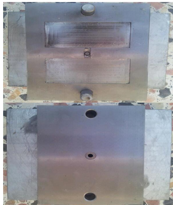
Fig. 1 The injection mold used for producing the specimens.
