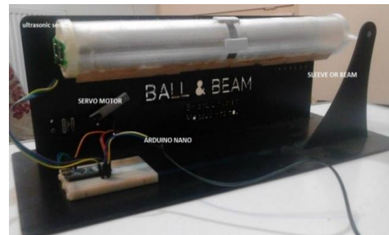
Fig. 4 Laboratory system for ball and beam control.
