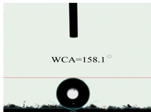
Fig. 3 Water contact angle image of 4% Silica-PDMS composite coated on the fabric.
