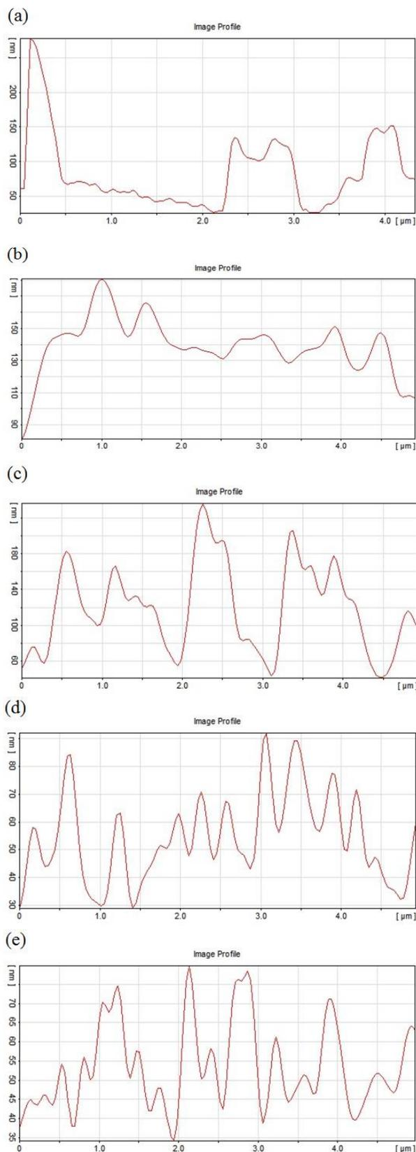
**Fig. 5** AFM roughness profiles of PDMS-Silica nano-composite coatings with: (a): 0.5, (b): 1, (c): 2, (d): 3 and (e): 4 wt% silica nano-particles.
