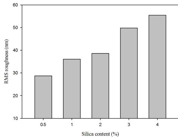
**Fig. 6** Roughness values of PDMS-Silica nano-composite coatings as a function of silica content.
