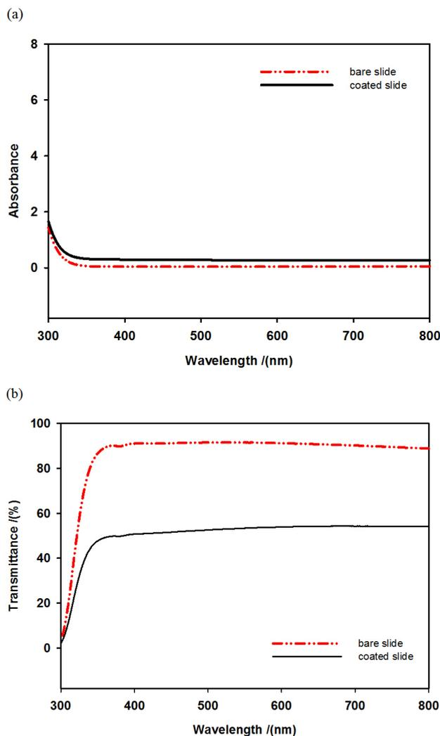
**Fig. 8** (a): Optical absorbance spectral values and (b): optical transmittance spectral values of bare glass slide and glass slide coated with 4% Silica-PDMS composite.
