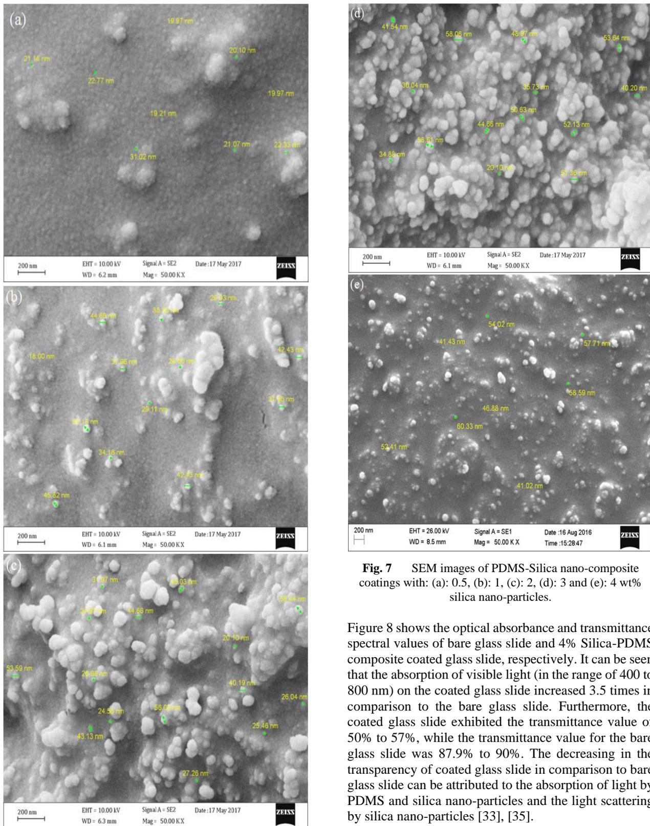
**Fig. 7** SEM images of PDMS-Silica nano-composite coatings with: (a): 0.5, (b): 1, (c): 2, (d): 3 and (e): 4 wt% silica nano-particles.
