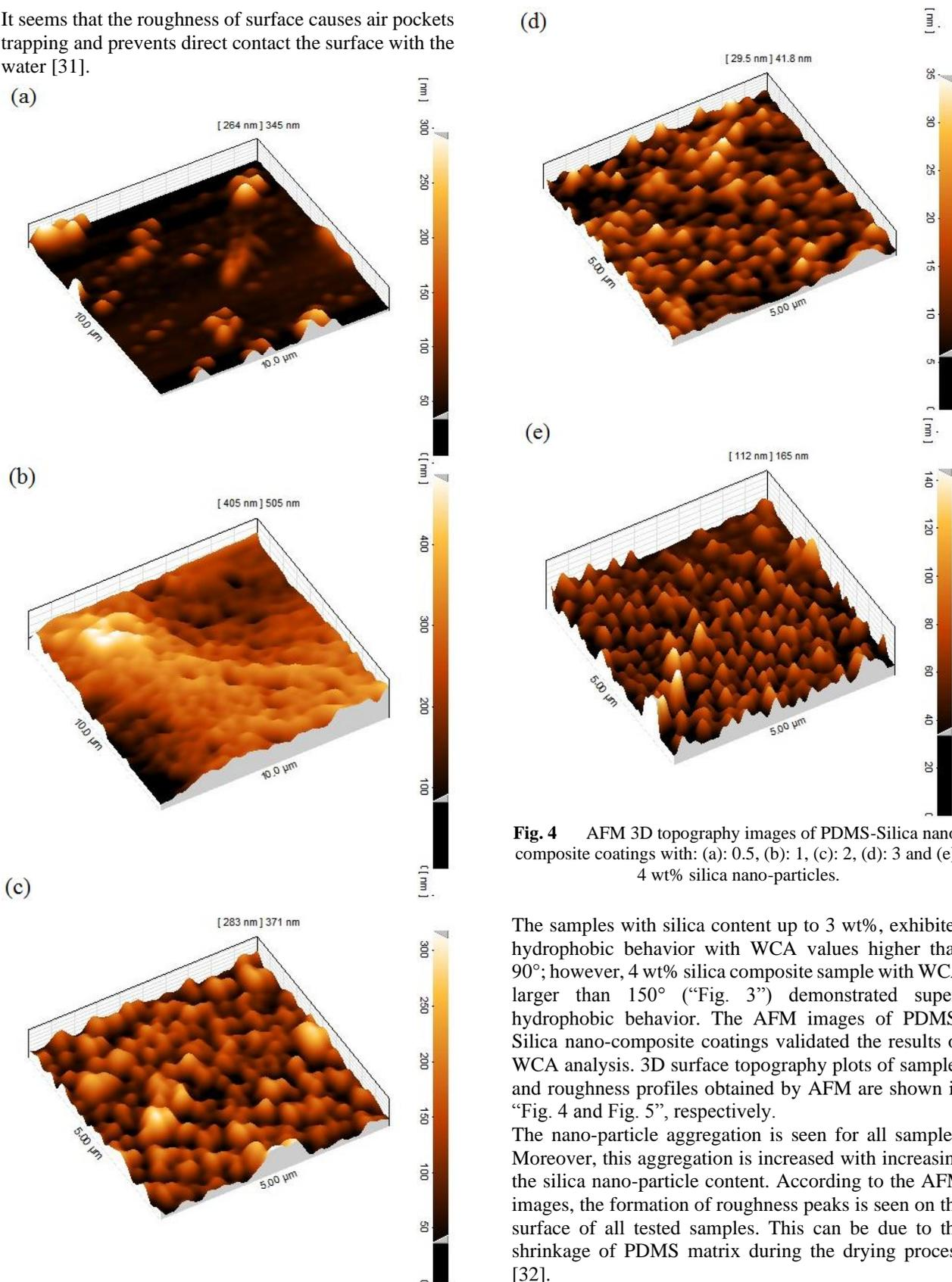
**Fig. 4** AFM 3D topography images of PDMS-Silica nano-composite coatings with: (a): 0.5, (b): 1, (c): 2, (d): 3 and (e): 4 wt% silica nano-particles.
