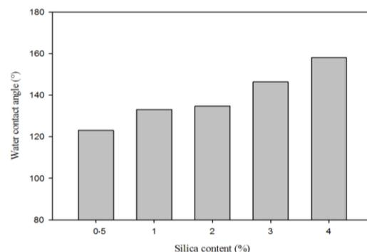
Fig. 2 Water contact angle values of PDMS-Silica nano-composites coatings as a function of silica content.
