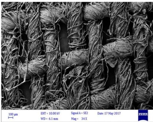
Fig. 1 SEM image of fibers structure in the fabric.
