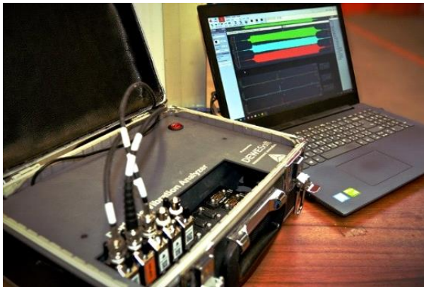
Fig. 5 The testing system with vibration sensors.
