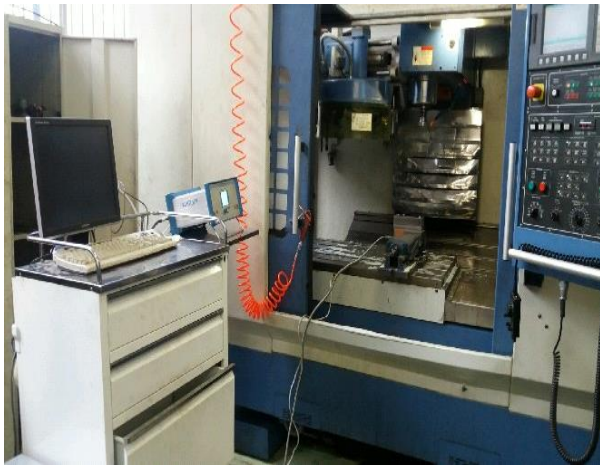
Fig. 4 The milling machine and dynamometer that are used in the test.
