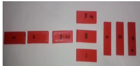
Fig. 18 Build product of all orientation of 0.3302 mm LT
