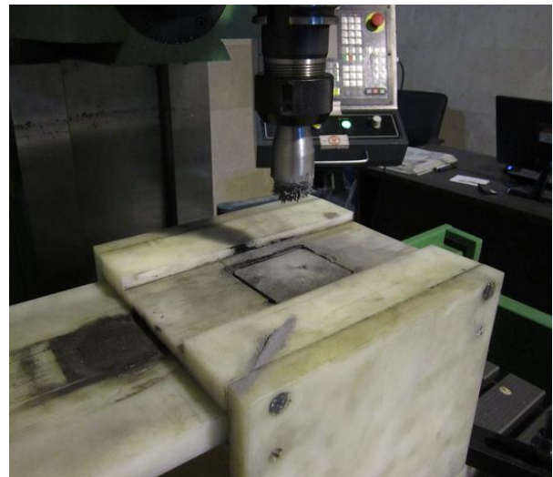
Fig. 4 Magnetic abrasive finishing process on IN718 surface
