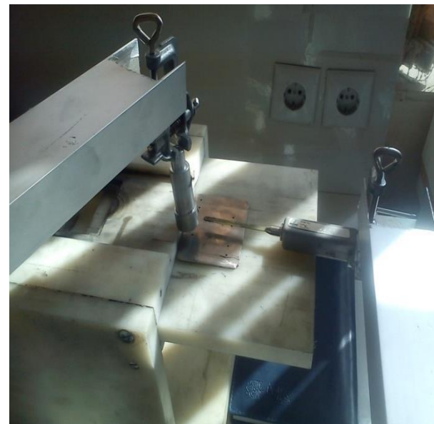
Fig. 1 Measuring procedure of magnetic flux density (mT) using gauss meter
