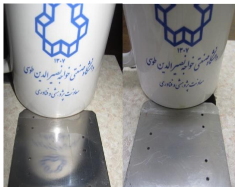
Fig. 13 Effect of MAF process on IN718 surface quality
