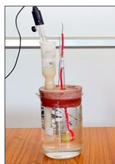
Fig. 2 (a) The components of an electrochemical cell for polarization test and (b) Assembly of an electrochemical cell
