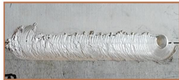
Fig. 2 Lateral flash in the joint FSW
