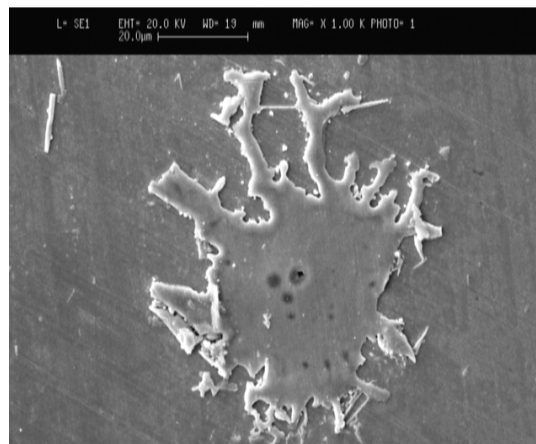
Fig. 2. Top surface morphology of fragmented and splashed splat collected at room temperature.
