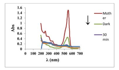
Figure 11.Photodegradation of RB on V<sub>2</sub>O<sub>5</sub>-ZnO/SiO<sub>2</sub> photocatalyst at pH=5 (under visible light).
