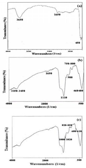
Figure 2. FT-IR spectra of (a) ZnO, (b) ZnO/SiO<sub>2</sub>, and (c) V<sub>2</sub>O<sub>5</sub> - ZnO/SiO<sub>2</sub> samples.
