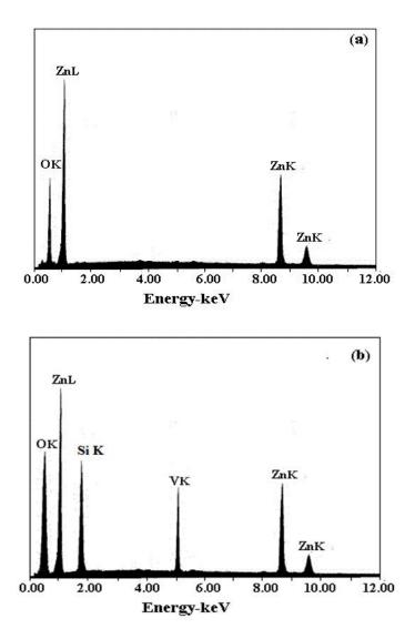
Figure 4. EDX spectra of (a) bare ZnO, and (b) V<sub>2</sub>O<sub>5</sub>- ZnO/SiO<sub>2</sub> nanoparticles.
