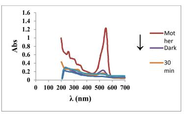
Figure 10. Photodegradation of RB on V<sub>2</sub>O<sub>5</sub>-ZnO/SiO<sub>2</sub> photocatalyst at pH=5.
