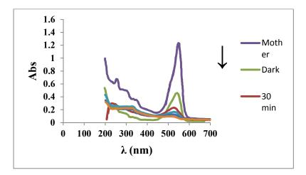
Figure 9. Photodegradation of RB on bare ZnO/SiO<sub>2</sub> photocatalyst at pH=6.
