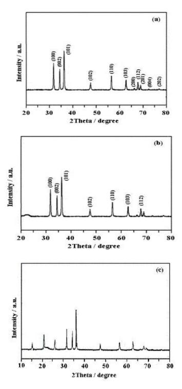
Figure 1. XRD patterns of (a) ZnO, (b) ZnO/SiO<sub>2</sub>, and (c) V<sub>2</sub>O<sub>5</sub> - ZnO/SiO<sub>2</sub> samples.
