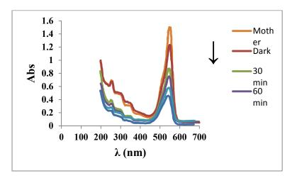
Figure 6.Photodegradation of RB on bare ZnO/SiO<sub>2</sub> photocatalyst at pH=3.
