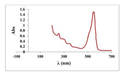
Figure 5. UV-Vis spectrum of Rhodamine B (10ppm).
