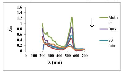
Figure 7.Photodegradation of RB on bare ZnO/SiO<sub>2</sub> photocatalyst at pH=4.
