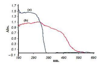
Figure 12. UV-Vis Diffuse Reflectance Spectra of (a) ZnO/SiO<sub>2</sub>, and (b) V<sub>2</sub>O<sub>5</sub>-ZnO/SiO<sub>2</sub> nanoparticles.
