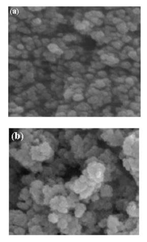
Figure 3. SEM images of (a) bare ZnO, and (b) V<sub>2</sub>O<sub>5</sub>- ZnO/SiO<sub>2</sub>nanoparticles.
