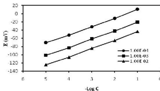
**Figure 2.** The effect of internal reference solution concentration on the electrode response.
