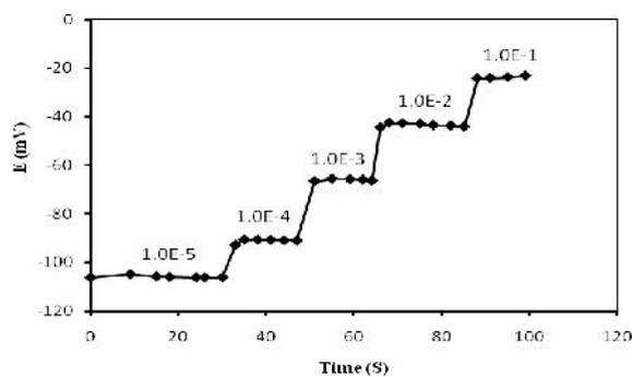
**Figure 3.** Dynamic response of chromium ion electrode for step changes in concentration of Cr(III)
