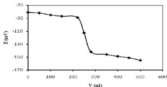
**Figure 5.** Potentiometric titration curve of  $1.0 \times 10^{-4}$  M Cr(III) solution (25 ml) with  $1.0 \times 10^{-2}$  M EDTA using the proposed sensor as an indicator electrode.
