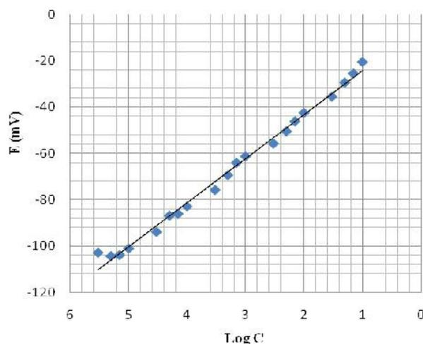
**Figure 4.** The calibration curve of the chromium ion-selective electrode.
