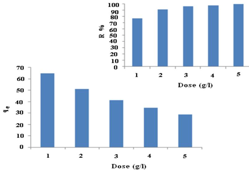
**Figure 4.** The effect of adsorbent amount, conditions: Ni<sup>2+</sup> initial concentration=100 mgL<sup>-1</sup>, pH= 8 and temperature=25 °C.
