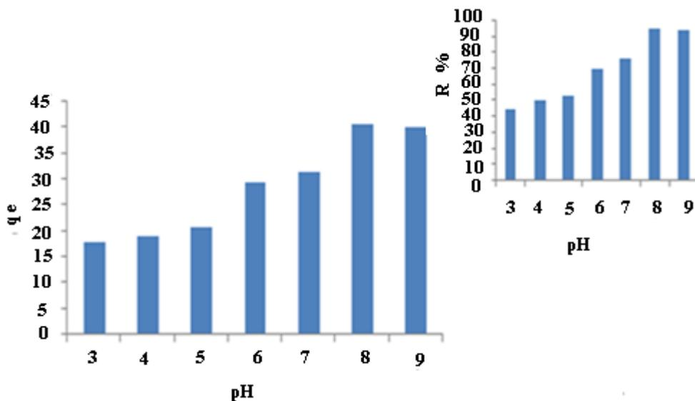
Figure 3. Effect of pH on Ni (II) removal; conditions: adsorbent dose=2 mg l<sup>-1</sup>, initial concentration=100 mg l<sup>-1</sup>, agitation time=180 min at 500 rpm and 25 °C.
