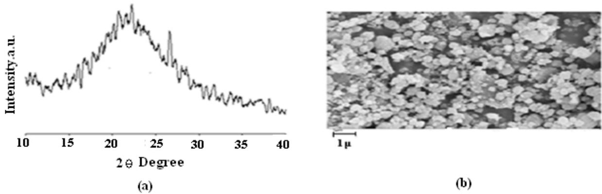
Figure 2. (a) XRD pattern of PLA at 600°C and (b) SEM PLA with leaching at 600°C.
