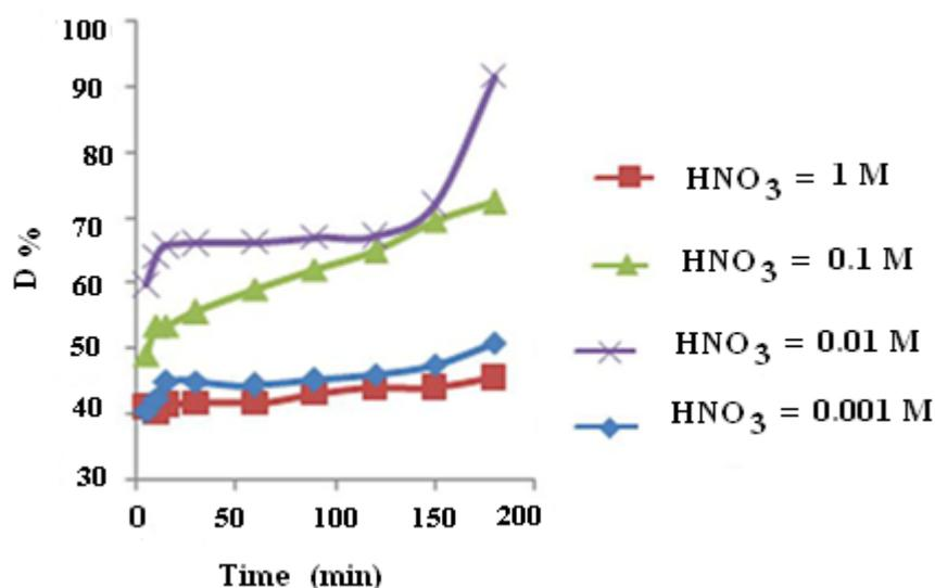
**Figure 5.** Desorption for Ni ions by PLA adsorbent; conditions: initial Ni<sup>2+</sup> concentration=1gL<sup>-1</sup>, pH= 8 and temperature=25 °C
