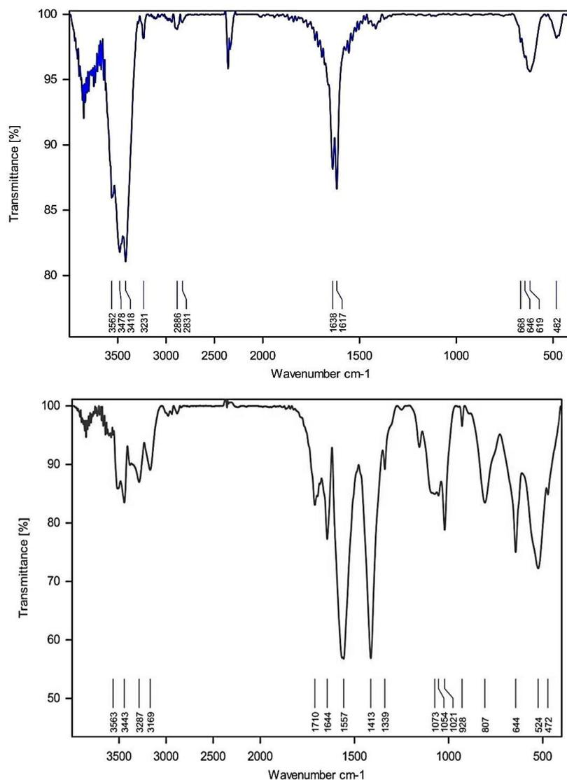
Figure 4. FT-IR spectrum of the prepared film: (blue line) CS/Cu; (Red line) PVPP/CS/Cu.
