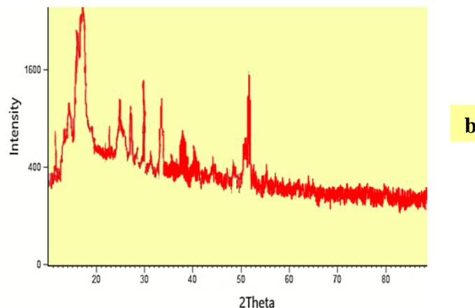
**Figure 3.** XRD patterns of *a*:PVPP/CS and *b*: PVPP/CS/Cu film.
