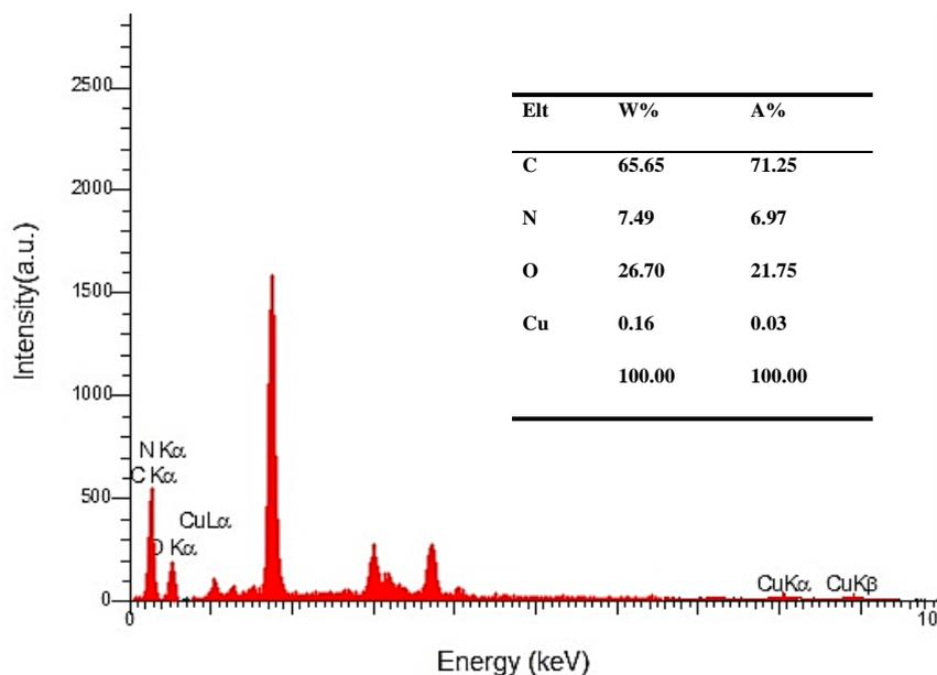
**Figure 2b.** EDS of PVPP/CS/Cu film.
