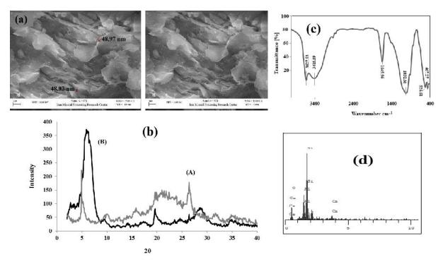
**Figure 1.** (a) SEM images (b) XRD patterns of the *Ghezeljeh* nanoclay are treated with ethylene glycol (A), Untreated (B). (c) FT-IR spectrum (d) EDX spectrum of untreated *Ghezeljeh* nanoclay.
