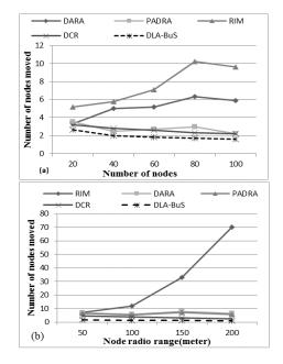
Figure 9: The number of nodes moved during the recovery, while varying (a) the network size (b) and radio range.
