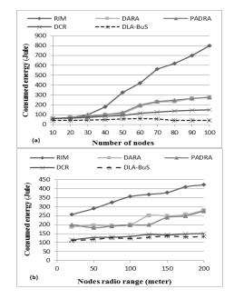
Figure 13: Percentage of consumed energy during the recovery, while varying (a) the network size and (a) radio range.
