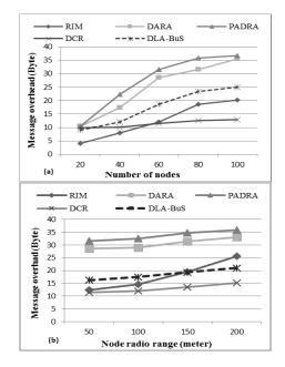
Figure 11: Message overhead during the recovery, while varying (a) the network size (b) and radio range.
