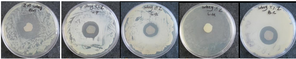
Fig. 1. Inhibition zones of Whey protein isolate films incorporated with 2% zataria multiflora Boiss. essential oil on Listeria monocytogenes (L.M), Bacillus cereus (B.C), Staphylococcus aureus (S.a), Escherichia coli O157: H7 (E.coli) and vibrio parahaemolyticus (V.P)
