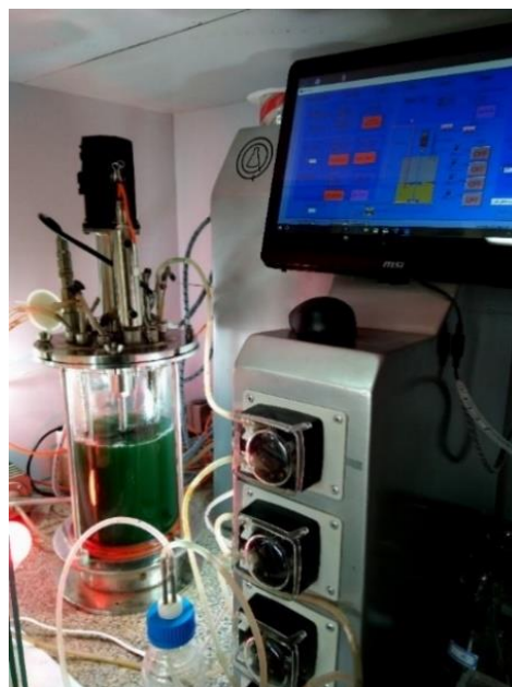
Figure 1- Stirred tank photobioreactor for cultivation Spirulina platensis
