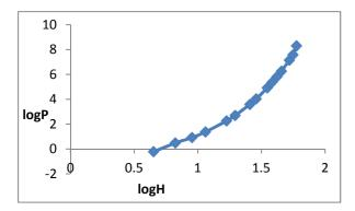
**Fig. 4**. Plots of the log H versus log P for  $(C_2-C_{20})$  monocarboxylic acids (without  $C_6, C_9, C_{12}, C_{17}$ ).
