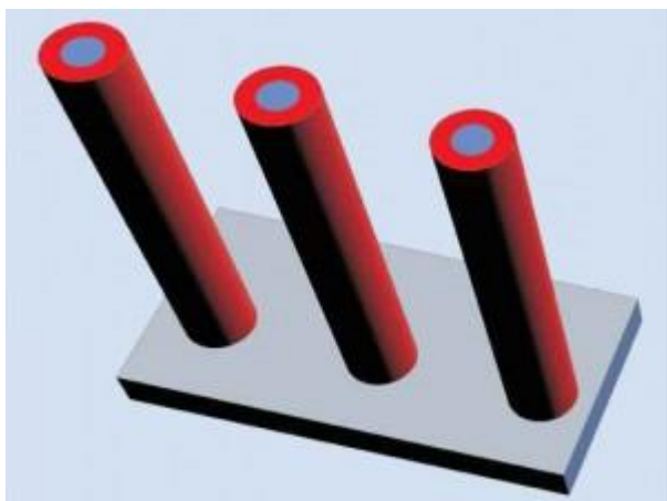
Fig. 2. This shows a layer of n-type silicon forming a shell around a p-type silicon core [8].
