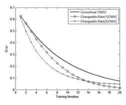
Fig.7. Error Comparison for different CMAC models.
