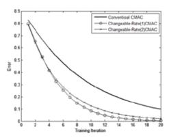
Fig. 5. Error Comparison for different CMAC models.
