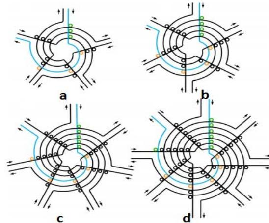
Fig.15. General structure of router with  $n$  ports; a)  $n=5$ , b)  $n=6$ , c)  $n=7$ , d)  $n=8$ [19]
