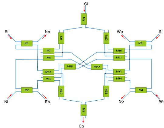
Fig20. 5x5 optical router based on Mach-Zehnder interferometer[4]
