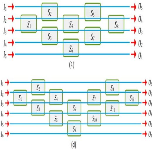
Fig18. N-Port non-blocking optical router based on MZI; a) n=3, b) n=4, c) n=5, d)n=6 [24]
