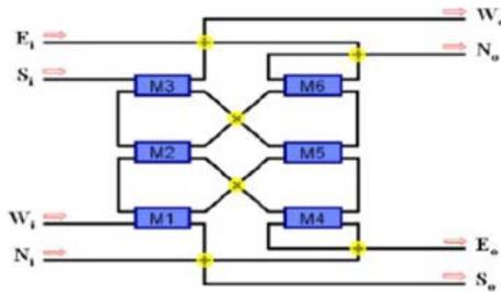
Fig16. Non-blocking 4×4 optical router based on Mach-Zehnder interferometer[21]
