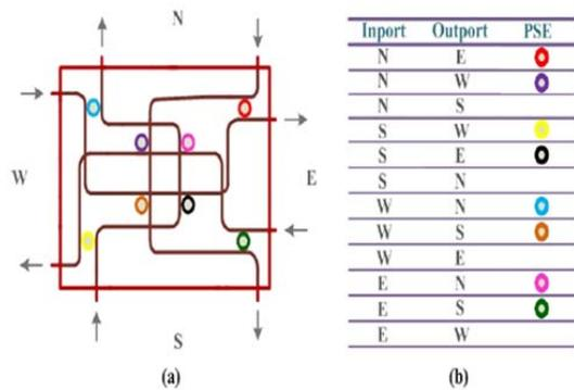
Fig17. a) 4×4 optical router based on Micro Ring Resonator b) Routing paths of the four-port optical router[22]
