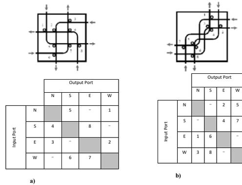
Fig10. Router with 4 non-blocking ports;
