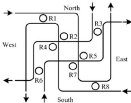
Fig.13. Non-blocking Four-ports optical router[17]
