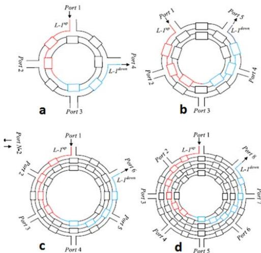
Fig23. Total structure of router with n ports; a) n=4, b) n=5, c) n=6, d) n=7[25]
