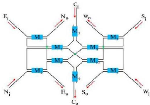
Fig19. 5x5 optical router based on Mach-Zehnder interferometer[23]
