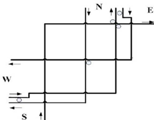
Fig27. Specific-purpose optical router under XY algorithm with 4-Port[3]
