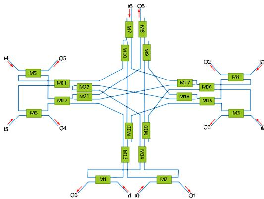
Fig22. 7x7 optical router based on Mach-Zehnder interferometer[20]
