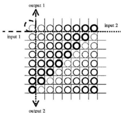
Fig6. The first basic architecture for optical routing with micro-ring resonators[10]
