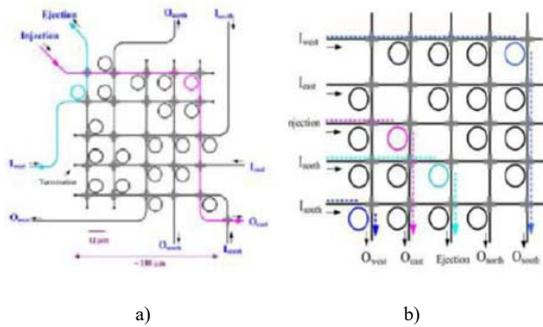
Fig.12. 5x5 non-blocking optical router; a) initial design, b) improved design [16]
