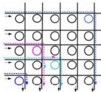
Fig11. Non-blocking optical router with 5 ports[15]
