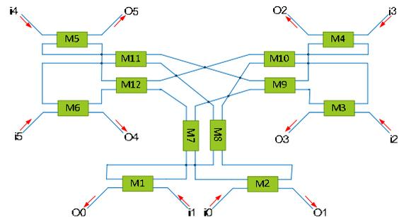
Fig21. 6x6 optical router based on Mach-Zehnder interferometer[20]
