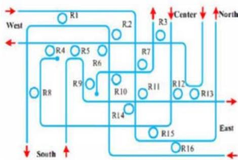
Fig.14. Non-blocking Five-ports optical router[18]
