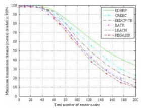
Fig5. Maximum transfer distance in total number of sensor nodes
