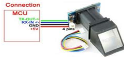
Fig.4. Fingerprint (R305) Architecture
