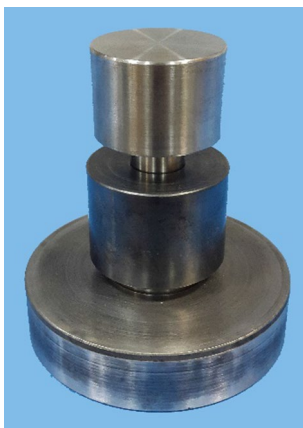
Fig. 1 Custom-made press mold designed for fabricating cylindrical tablets
