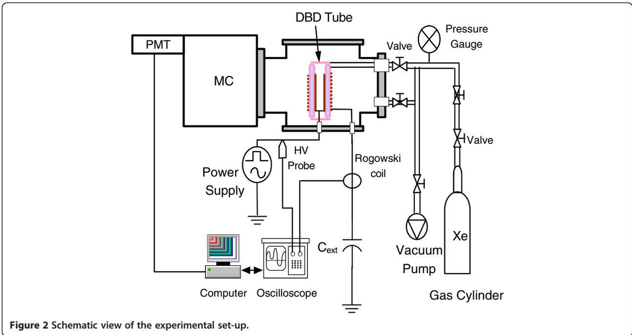
**Figure 2** Schematic view of the experimental set-up.
