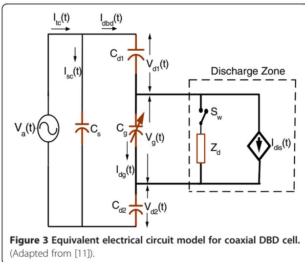
**Figure 3** Equivalent electrical circuit model for coaxial DBD cell. (Adapted from [11]).
