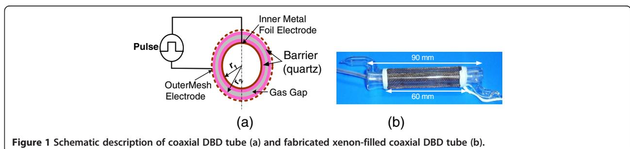
**Figure 1** Schematic description of coaxial DBD tube (a) and fabricated xenon-filled coaxial DBD tube (b).
