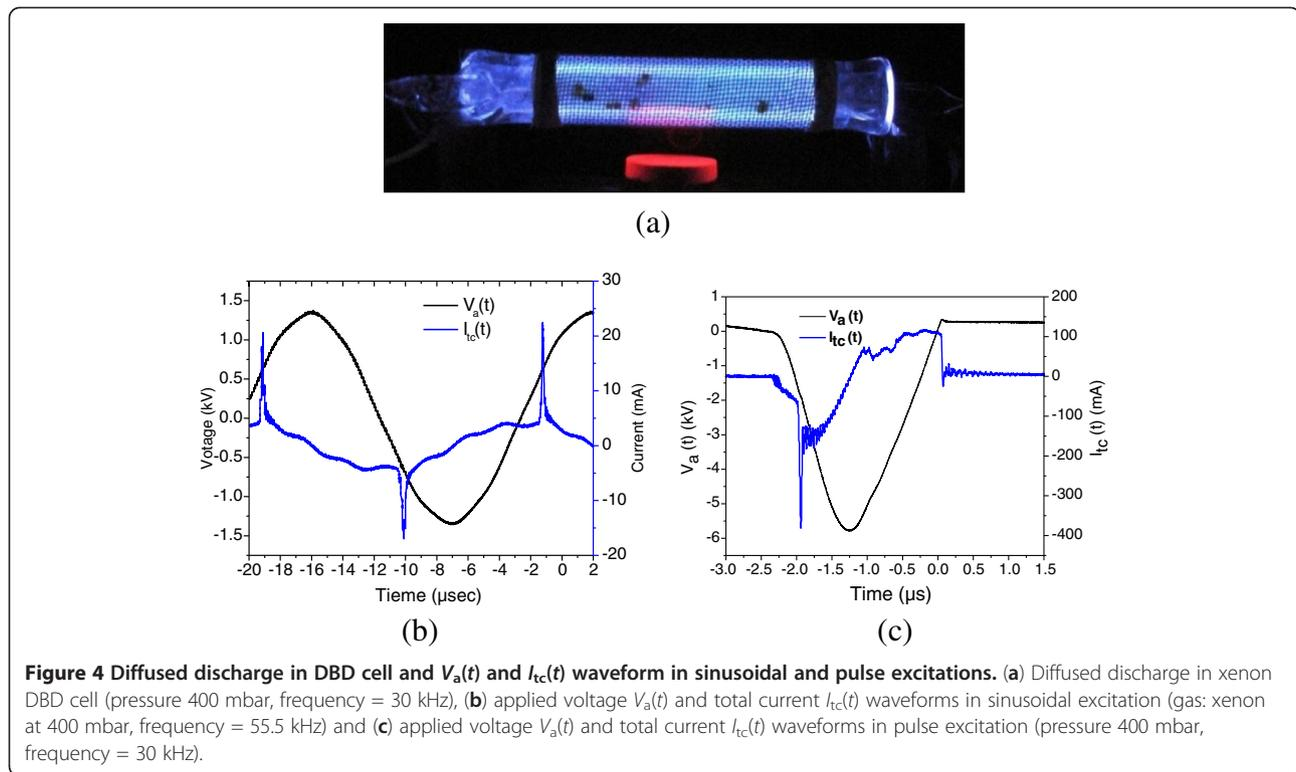
Japan; exposure time 25 ms) for the xenon coaxial DBD tube. The image indicates that the diffuse discharge covers the entire surface of the electrodes. Figure 4b,c shows the total current trace together with the applied voltages for sinusoidal and unipolar pulse excitations, respectively, where the discharge current waveform having only a few numbers of current pulses with a nanosecond order is superimposed on the total current.
