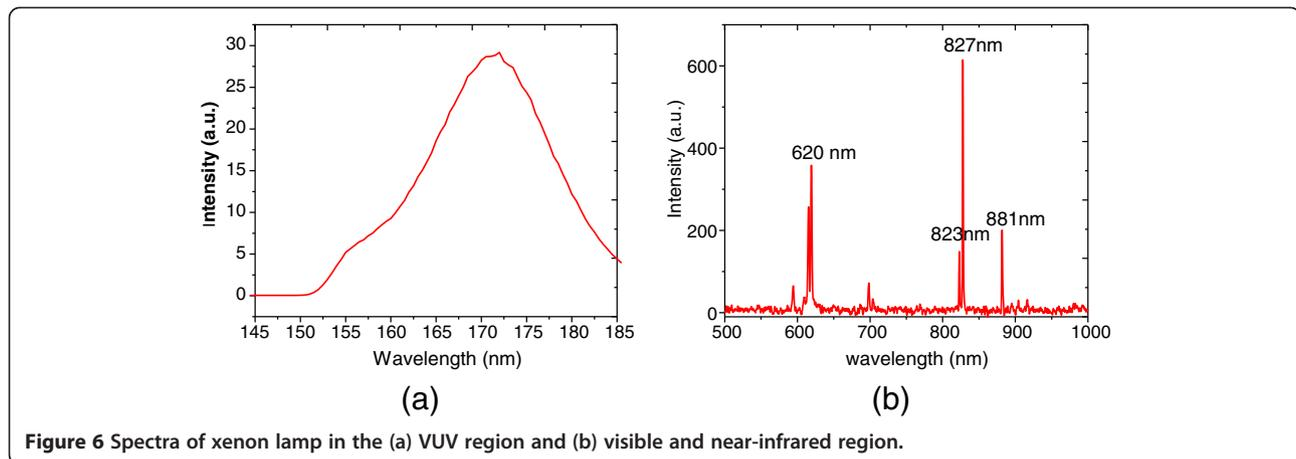
vibrationally relaxed excimer molecules  $Xe_2^*(0_u^+, \nu \approx 0)$  and  $Xe_2^*(1_u, 0_u^-, \nu \approx 0)$  decay subsequently through radiative processes by the following reactions and generate wavelength 172 nm in the DBD source [16]:
