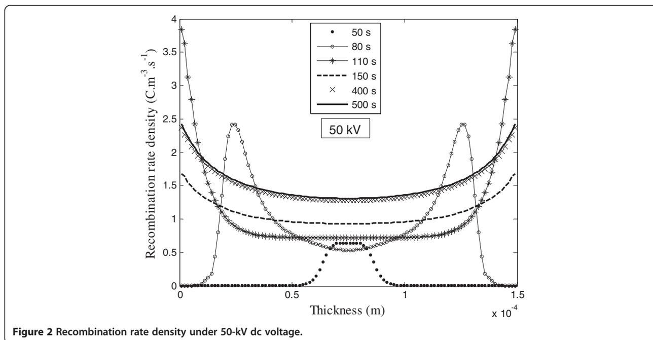
This figure indicates that the recombination rates are confined near the anode and the cathode, respectively. This is due to the electron and hole packets which propagate respectively towards the opposite electrode and recombine with trapped holes and trapped electrons which are located close to the anode and the cathode, respectively, as seen in Figure 5a,b.
