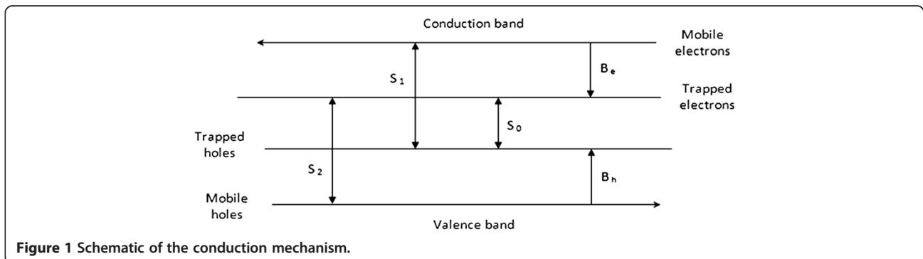
**Figure 1** Schematic of the conduction mechanism.
