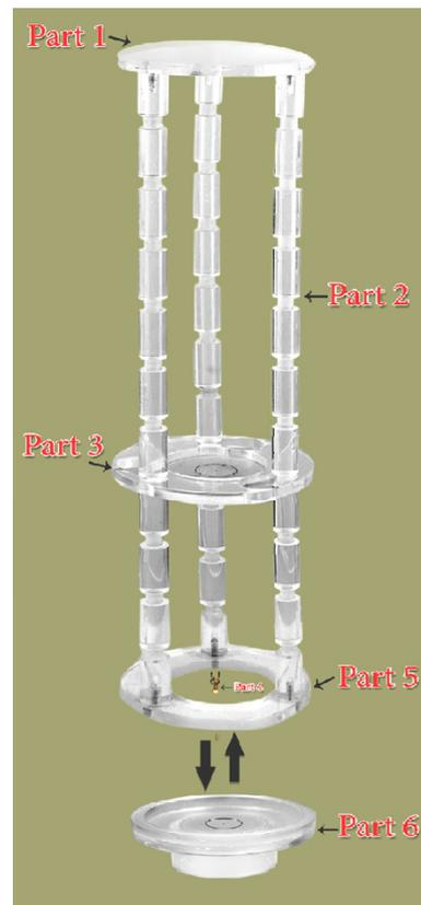
**Fig. 1** Homemade Plexiglass holder
