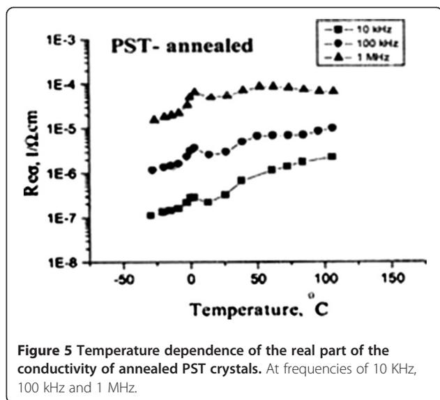
the annealing and doping effects can shift the phase transition to higher temperatures. The conductivity,  $Re\sigma$ , increases with increasing temperature for all investigated samples.
