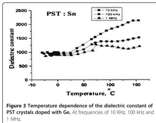
the perovskite, and the crystal lattice should be destroyed in the vicinity of the incorporated Ge atoms, thus affecting the ferroelectric properties.
