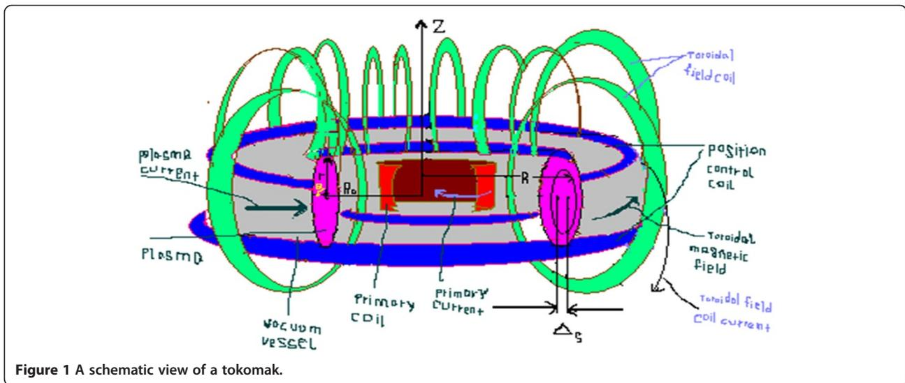
Figure 1 A schematic view of a tokamak.
