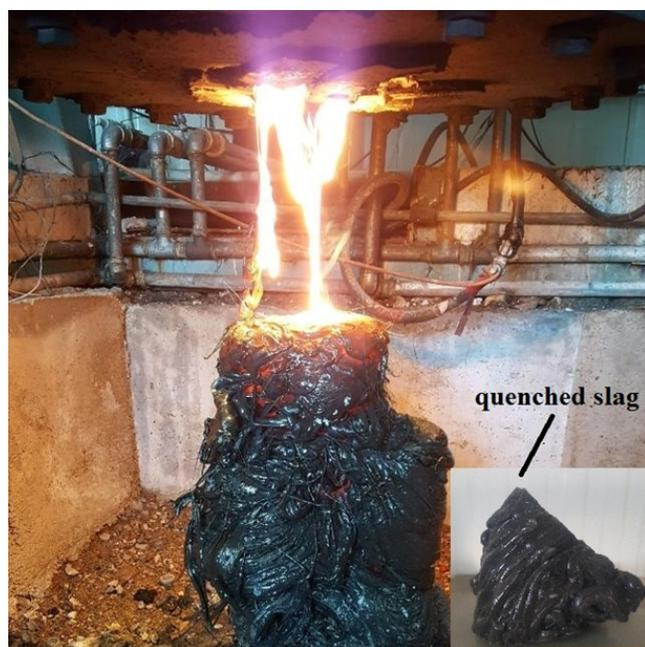
**Figure 4.** Molten material leaking from the furnace bottom.
