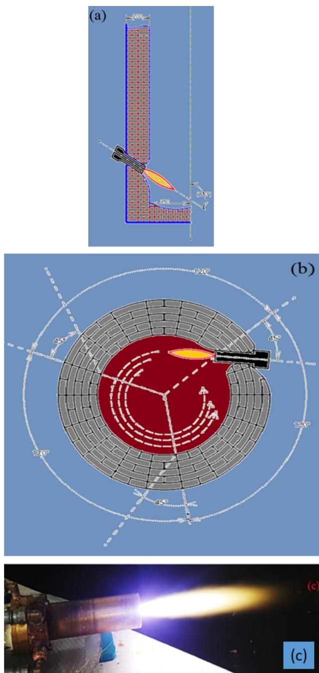
**Figure 3.** (a) Position of the plasma torches respect to furnace axis, (b) Position of the plasma torches respect to furnace circumference, (c) Plasma torch in operation.
