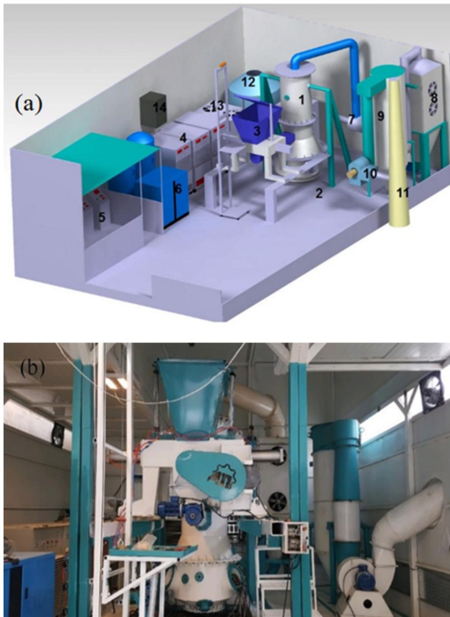
**Figure 1.** (a), (b) System setup: 1- main shaft furnace, 2- plasma torch, 3- feeding system, 4- power supplies, 5- control room, 6- air compressor, 7- after-burner, 8- water quench, 9- wet scrubber, 10- jet fan, 11- stack, 12- water reserve, 13- chiller, 14- Air purification system.
