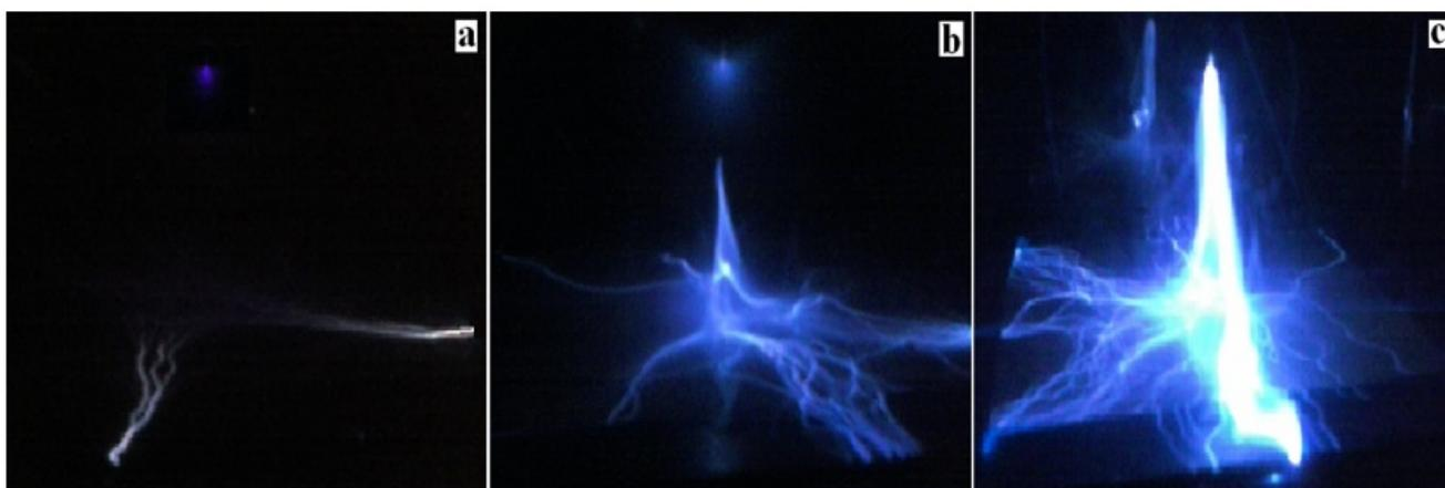
**Figure 2.** Photographs showing the evolution of the operation of a negative dielectric-barrier corona. The dielectric barrier is a polymer film.
