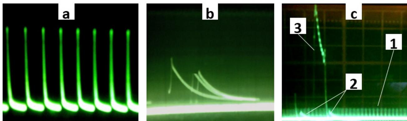
**Figure 3.** Current pulse oscillograms: (a) negative corona with dielectric barrier ( $I=184 \mu\text{A}$ ,  $t=40 \mu\text{s}$ ); (b) low-current surface discharge ( $I=44 \mu\text{A}$ ,  $t=1.2 \text{ ms}$ ); (c) (1) negative corona current pulses; (2) surface discharge current pulses; (3) streamer discharge current pulse ( $I = 1.4 \text{ mA}$ ,  $t = 0.3 \text{ ms}$ ).
