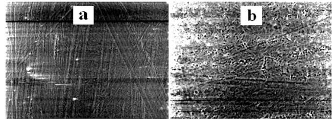
**Figure 5.** Photomicrographs of the surface of (1)initial and (2)modified PTFE. Magnification, 1500.
