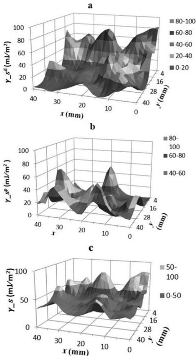
**Figure 4.** Influence of the character of current spreading on the surface energy of the modified PTFE film: (a)dispersive component, (b)polar component, and (c)total surface energy.
