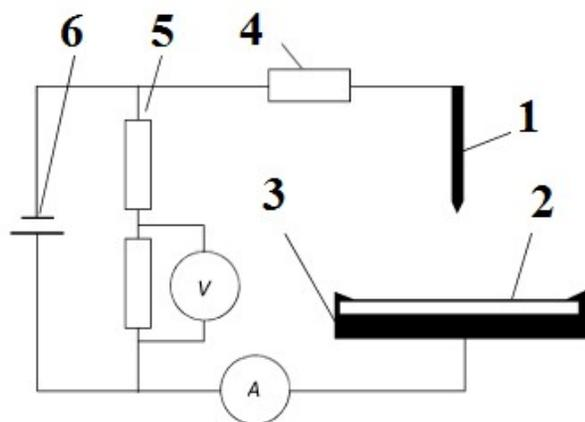
**Figure 1.** Schematic of the experimental setup: (1) point electrode, (2) plane electrode, (3) dielectric barrier made of polymer film, (4) ballast, (5) voltage divider, and (6) power supply.
