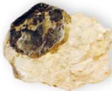
Figure 1. Macroscopic image of the layered crystalline structure of mica, illustrating its platelet-like morphology, which underpins its high thermal stability and effectiveness as a physical barrier in heat-resistant applications [7].
