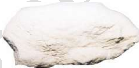
Figure 2. Macroscopic view of dolomite mineral, showing its massive texture and mineral structure, which serve as a source of endothermic reactions and refractory phase formation in heat-resistant systems [12].
