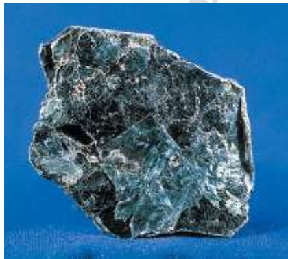
Figure 3. Macroscopic view of vermiculite mineral with a layered structure and platelet-like appearance, highlighting its high thermal expansion capability and its ability to form porous insulating layers at elevated temperatures [17].
