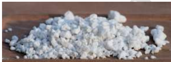
Figure 4. Macroscopic view of expanded perlite, showing its porous granular structure and low density, which make it an effective material for thermal insulation and heat transfer reduction [21].
