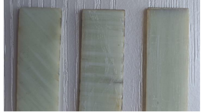
Fig .1. Unidirectional GFRP sheets in 3 different angles: (a) 45, (b) 90, and (c) 0
