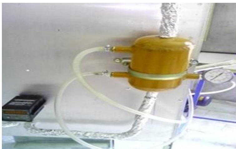
Fig. 2. Image of a fluidized bed reactor.
