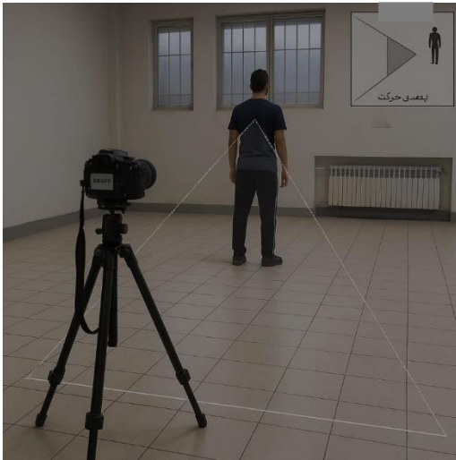
Fig 3. Camera layout, field of view, and line-of-sight relative to the movement execution area.
