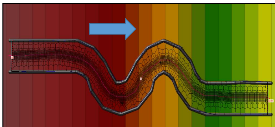
Fig 3. Meshing and geometry of the hydraulic model
