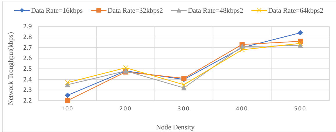
Fig 8. Network throughput vs node density for various data rates
