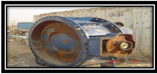
Figure (10) A view of the destruction of butterfly valve due to lack of proper connection
