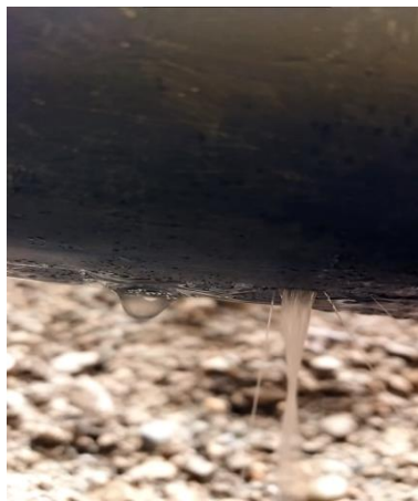
b) Hole damage in polyethylene pipe
