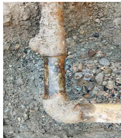
a) Crack damage in steel pipe
