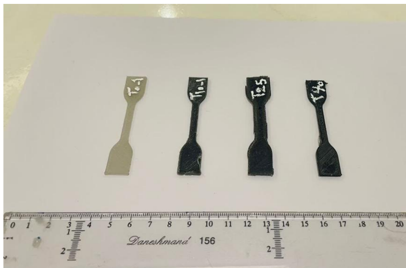
Figure 1. The printed dog-bone specimens
