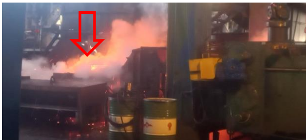
Fig. 2 Cooling using water in the descaling section of the rolling process to remove oxide scales from the surface of rolled metals
