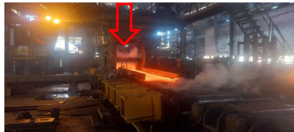
Fig. 3 Use of water in the rolling stand section for cooling the rolling mill roller
