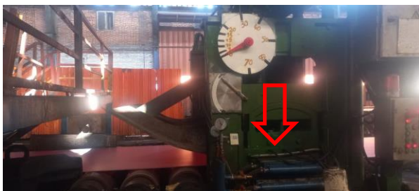
Fig. 4 Cooling the scarfing machine using water to remove waves, control thickness, and reduce defects
