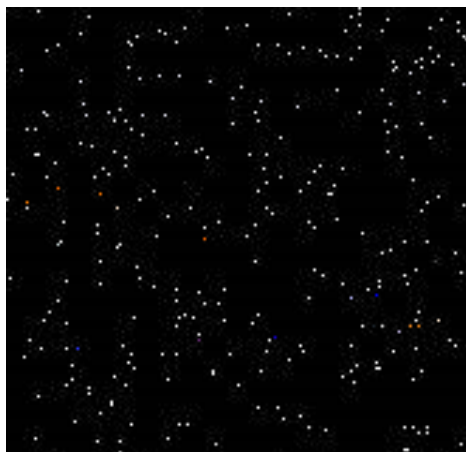
Fig4. Spreading platinum on the surface of the polyaniline modified electrode
