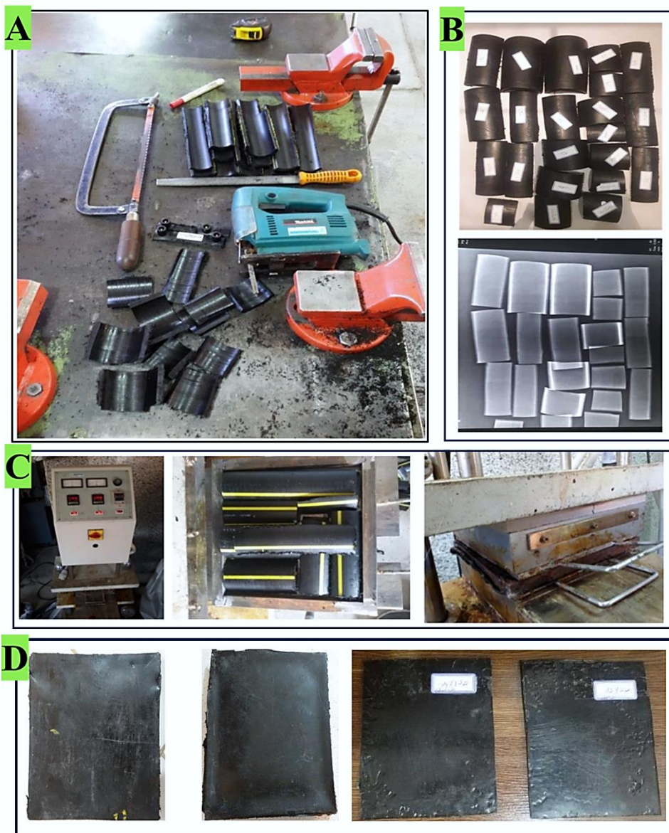
Fig. 4 Pipe cutter and coupler (A), using radiography to ensure that there is no remaining copper wire in the cut parts of the coupler (B), preparing the sample for pressing in the hot press machine (C), pressed samples of coupler and polyethylene pipe (D)
