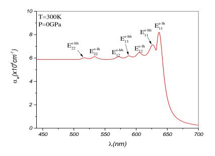
Fig. 12. Optical absorption versus wavelength for InGaN/GaN MQW solar cell.
