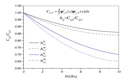
Fig. 3. Normalized overlap of the electron-hole wave functions versus hydrostatic pressure for InGaN/GaN MQW solar cell.
