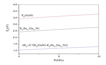
Fig. 1. Bandgaps energy of InGaN, GaN, and conduction band offset of InGaN/GaN MQW solar cell as a function of pressure.
