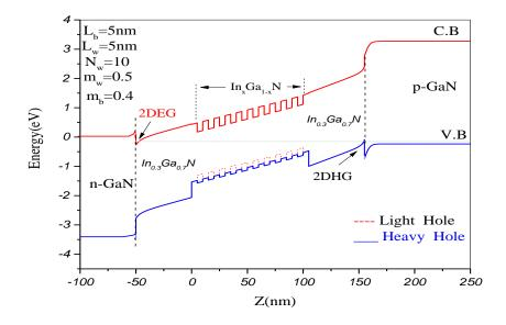
**Fig. 2**. The conduction (C.B) and valance (V.B) bands energy of InGaN/GaN MQW solar cell as a function of the distance under different hydrostatic pressure.
