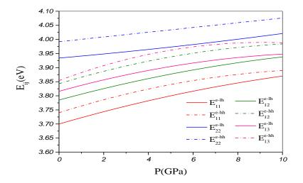
**Fig. 10.** Transition energy as a function of hydrostatic pressure at subband adage  $(k_{\parallel} = 0)$  for *InGaN / GaN* MQW solar cell. In which heavy hole (dashed line) and light hole (solid line) are considered.
