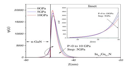
**Fig. 5.** The first subband electron waves function versus the distance for the  $GaN / In_{0.3}Ga_{0.7}N$  MQW solar cell under different hydrostatic pressures. The inset indicates the electron wave function impenetrate to the GaN barrier.
