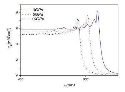
Fig. 13. Quantum well optical absorption versus wavelength under different hydrostatic pressures for *InGaN/GaN* MQW solar cell.
