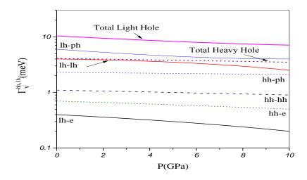
**Fig. 7.** Valance band linewidths as a function of hydrostatic pressure at subband adage  $(k_{\parallel} = 0)$  for *InGaN / GaN* MQW solar cell. In which all the scattering of holes with other holes (hh-hh, lh-lh), phonons (lh-ph, hh-ph) and with other electrons (e-hh, e-lh) are considered.
