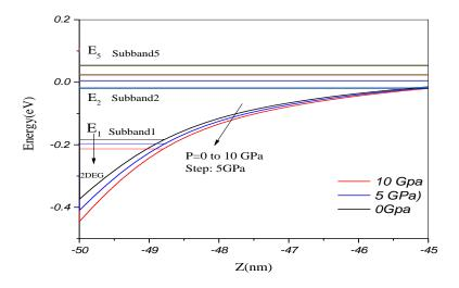
Fig. 4. The quantum well conduction band and subband of energy as a function of the distance under different hydrostatic pressures.
