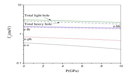
**Fig. 6.** Conduction band linewidths as a function of hydrostatic pressure at subband adage  $(k_{\parallel} = 0)$  for *InGaN / GaN* MQW solar cell. In which all the scattering of electrons with other electrons(e-e), phonons(e-ph), light holes(e-lh) and heavy hole(e-hh) are considered.
