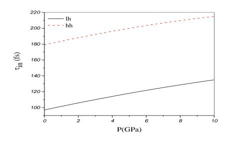
**Fig. 8.** Intraband relaxation time as a function of hydrostatic pressure at subband adage  $(k_{\parallel} = 0)$  for *InGaN / GaN* MQW solar cell. In which heavy hole (solid line) and light hole (dashed line) are considered.
