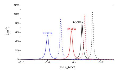
**Fig. 11.** Light hole (solid line) and heavy hole (dashed line) Lorentzian function versus of the energy difference  $(E - E_{11})$  under different hydrostatic pressures for *InGaN / GaN* MQW solar cell. In which the energy transition between the first subbands of electron energy levels with holes are considered.
