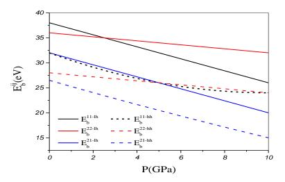
Fig. 9. Exciton Binding energy of heavy holes and light holes as a function of hydrostatic pressure for InGaN/GaN MQW solar cell.
